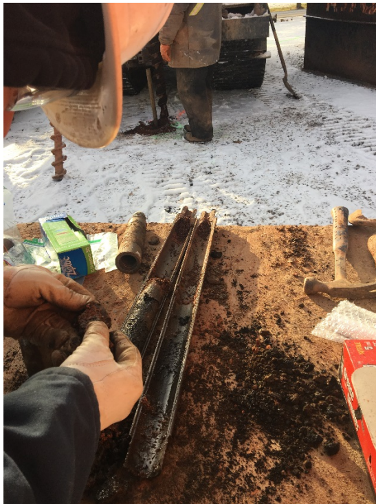
Photo 4 Geotechnical assessment of soil in split spoon from MW-12.
