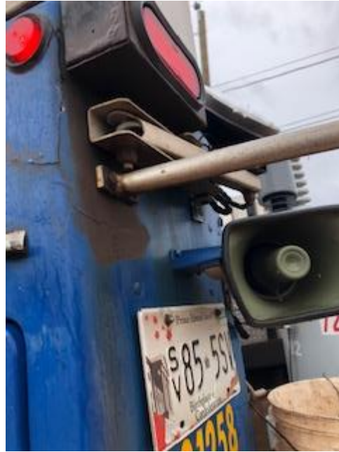
Truck 12-12-58 Corrosion at back of truck
