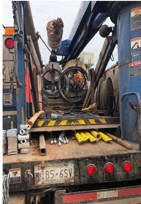
Truck 13-12-56 Corrosion of bed liner and false floor
