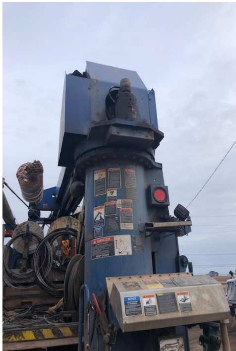
Truck 13-12-56 Turret for digger/derrick and control station
