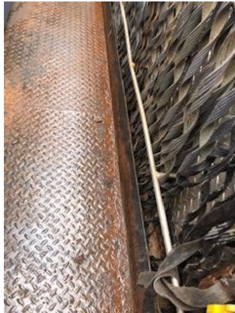
Truck 12-12-58 Corrosion holes through bed liner
