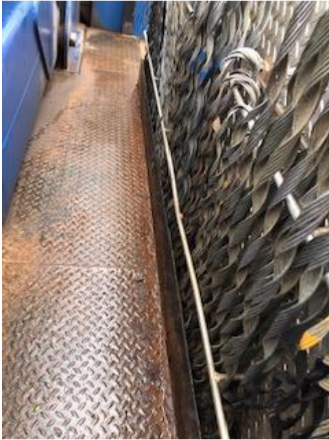
Truck 12-12-58 Corrosion of truck bed liner
