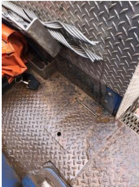
Truck 12-12-58 Corrosion/metal scaling in truck bed liner
