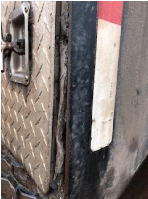
Truck 12-12-58 Corrosion around tool compartments
