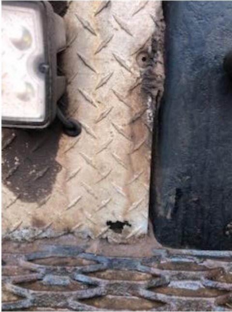
Truck 12-12-58 Corrosion / holes at tailgate
